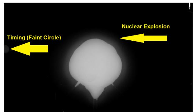
**Fig. 1.** An example timing mark
