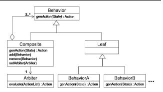
Fig. 3 Class diagram for the Unified Behavior Framework.
