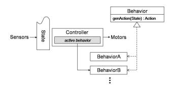
Fig. 2 Strong encapsulation of reactive behaviors allows the controller to change its active behavior during execution.
