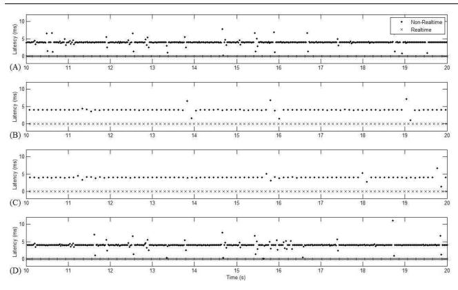
Fig. 7 Observed latency for (a) the laser driver; (b) the obs\_avoid behavior; (c) the rt-ubf controller; and (d) the robot driver.
