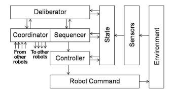
Fig. 5 The deliberative subsystem of HAMR will be preempted by the low-level controller and sensor subsystem.
