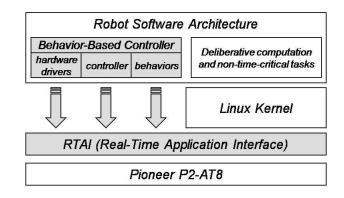
Fig. 1 Real-time tasks by pass Linux and run on the RTAI scheduler.
