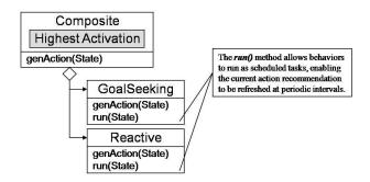
Fig. 4 Behavior structure formed from a goal-seeking element and a reactive element joined by a highest activation arbiter.
