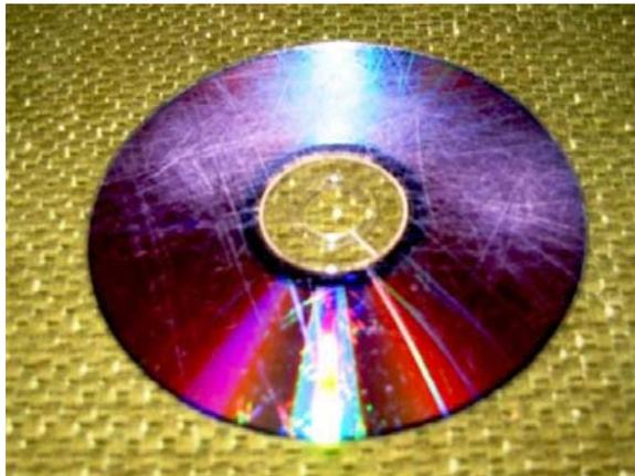
**Figure 3: Severely damaged DVD disk**
