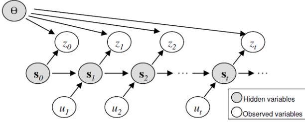
Fig. 1. SLAM as a DBN. Controls  $u_t$  and measurements  $z_t$  are observed at each time  $t$ , as vehicle poses  $s_t$  and a single map  $\Theta$  are hidden [7].
