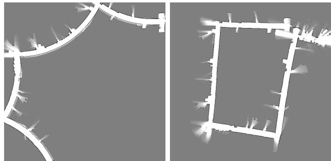
Fig. 5. Maps produced from LIDAR scans using odometry (left) and using the MINS path (right)
