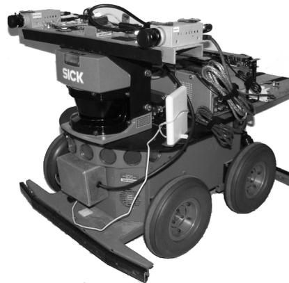
Fig. 3. The P2-AT8 vehicle with cameras and IMU above the LIDAR.
