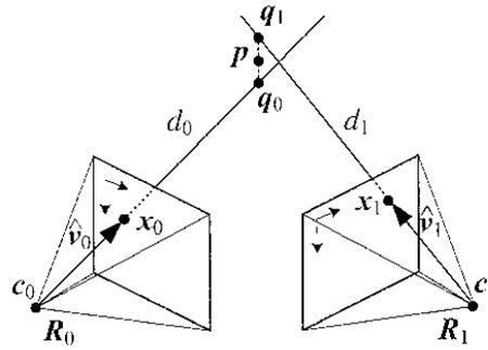
Fig. 5. 3D point triangulation [10]. Point  $p$  is estimated using rays traced from the centers of camera at  $R_1c_1$  and  $R_2c_2$ .
