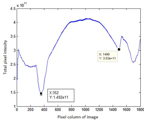
Fig. 7. A summary of pixel intensities by column. The low points on either side represent where the best area to crop the images would be.
