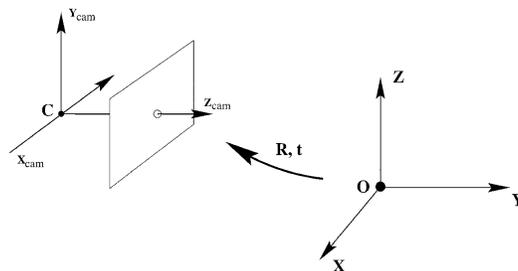
Fig. 4. The Euclidean transformation between world and camera coordinate frames is comprised of rotation ( $\mathbf{R}$ ) and translation ( $\mathbf{t}$ ) [8].
