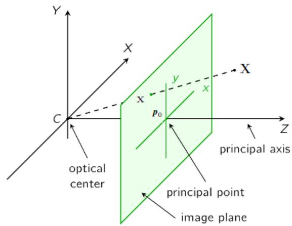
Fig. 3. The pinhole camera model.
